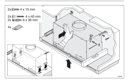
When fitting the DA 3590 in a 900 mm wide housing unit, the retaining brackets supplied are used to align the cooker hood and provide additional support.
